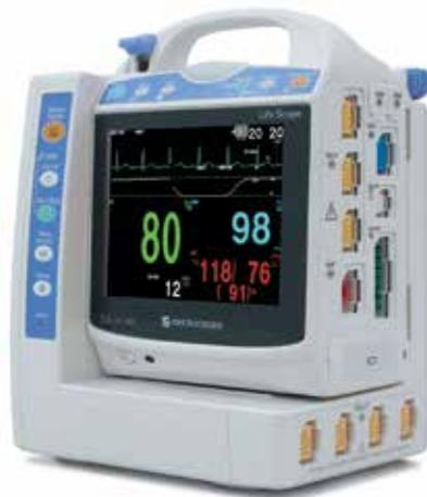
One additional benefit of the Data Acquisition Unit is that it can be extended via an umbilical cord to be located on a bed rail, gurney or IV pole next to the patient. This alleviates the hassles associated with cable management at the bedside. Since the Data Acquisition Unit contains user function keys, it can be placed on either side of the patient for optimal clinical workflow efficiency.
